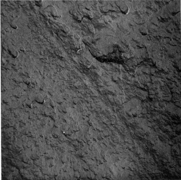
Fig. 1. Polyblend: PVC/NBR = 70/30. Mixing temperature: 275°F. Mixing time: 10 min. Replica: on cut section.
