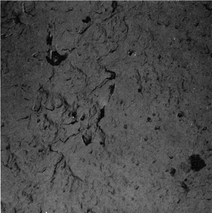
Fig. 4. Polyblend: PVC/NBR = 70/30. Mixing temperature: 300°F. Mixing time: 10 min. Replica: on cut section.
