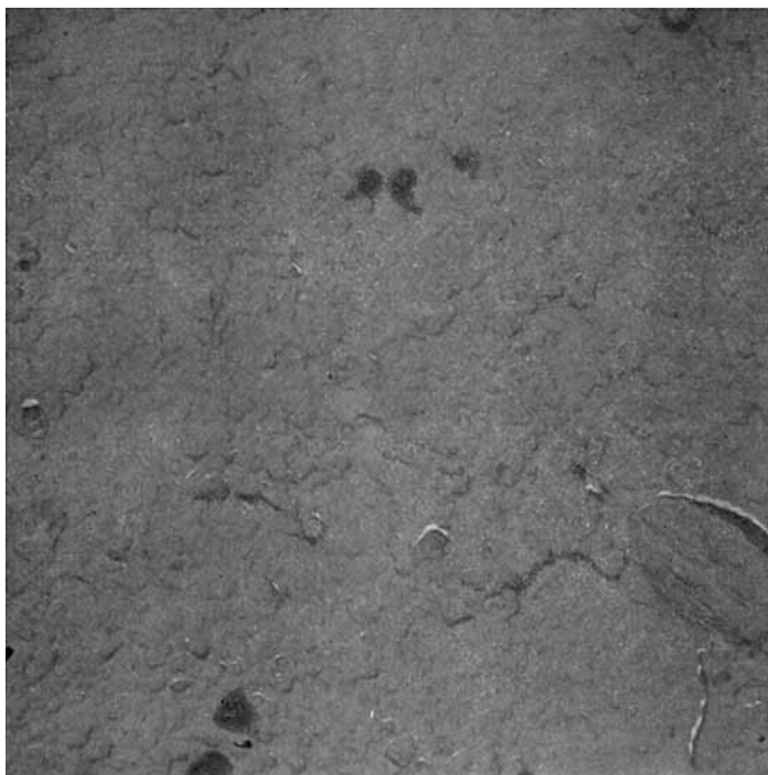
Fig. 20. Polyblend: PVC/NBR = 88/12. Mixing temperature: 300°F. Mixing time: 10 min. Replica: on cold-fracture section perpendicular to the calendaring direction.
