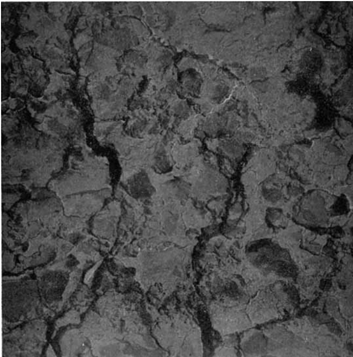
Fig. 23. Polyblend: PVC/NBR = 88/12. Mistron vapor: 5%. Mixing temperature: 300°F. Mixing time: 10 min. Replica: on cold-fracture section parallel to the calendaring direction.
