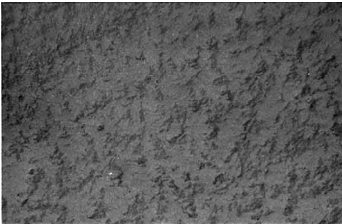
Fig. 29. Polyblend: PVC/NBR = 70/30. Mixing temperature: 300°F. Mixing time: 10 min. Replica: on cut section of a prestrained specimen.
