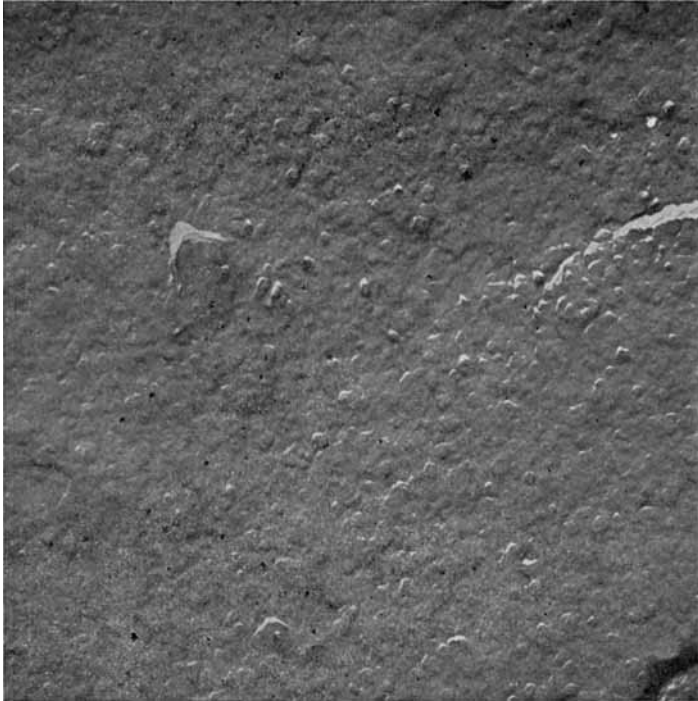
Fig. 14. Polyblend: PVC/NBR = 80/20. Mixing temperature: 300°F. Mixing time: 10 min. Replica: on cold-fracture section perpendicular to the calendering direction.
