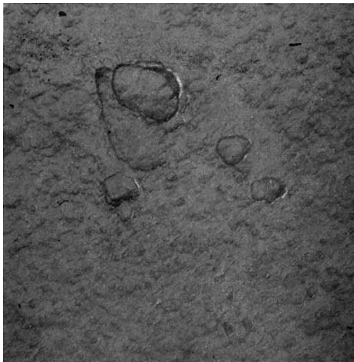
Fig. 19. Polyblend: PVC/NBR = 88/12. Mixing temperature: 300°F. Mixing time: 10 min. Replica: on cold-fracture section parallel to the calendaring direction.
